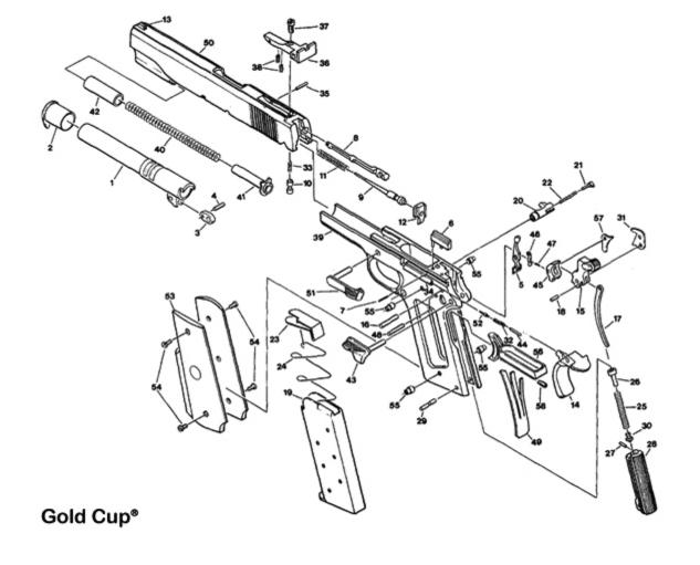
1: BARREL 2: BARREL BUSHING 3: BARREL LINK 4: BARREL LINK PIN 5: DISCONNECTOR 6: EJECTOR 7: EJECTOR PIN 8: EXTRACTOR 9: FIRING PIN 10: FIRING PIN PLUNGER 11: FIRING PIN SPRING 12: FIRING PIN STOP 13: FRONT SIGHT 14: GRIP SAFETY 15: HAMMER 16: HAMMER PIN 17: HAMMER STRUT 18: HAMMER STRUT PIN 20: MAGAZINE CATCH 21: MAGAZINE CATCH LOCK 22: MAGAZINE CATCH SPRING 25: MAIN SPRING 26: MAIN SPRING CAP
